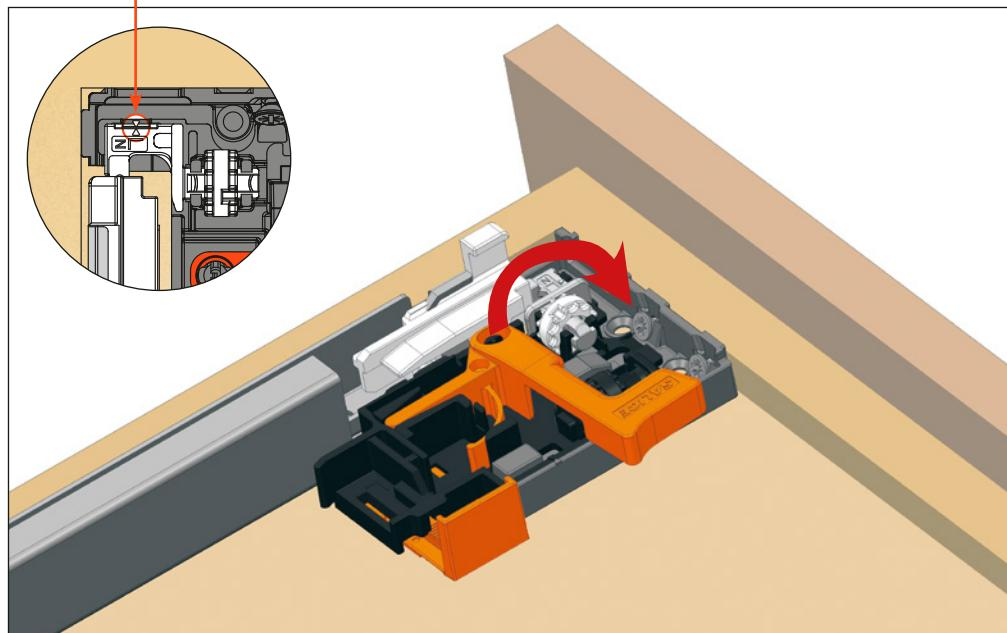
Rotate the white wheel towards the back of the drawer to adjust right.
