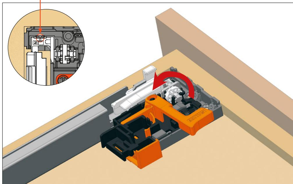
For side adjustment, it is recommended that both the adjusters on the clips are in the same direction, in order to maintain the correct alignment and function of the runners.
