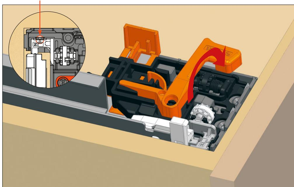
Rotate the black wheel towards the outside of the drawer to increase the gap between the front and the side.
